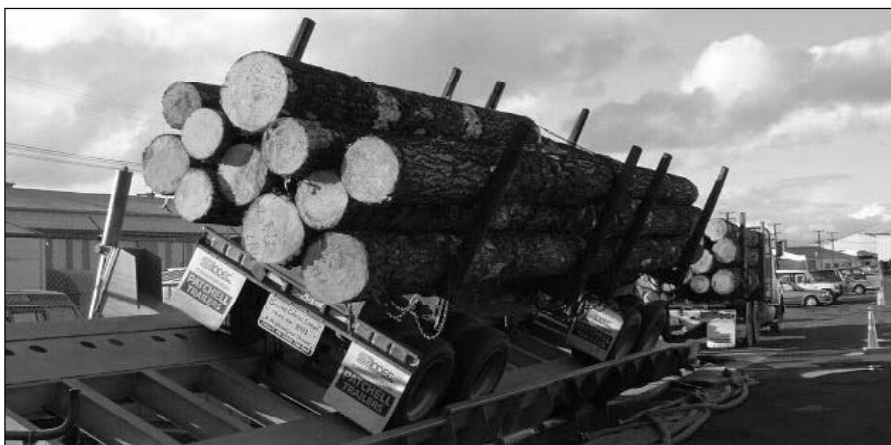
Trials showed lower, double packet trailer loads were 50 per cent more stable than shorter, single packet loads
