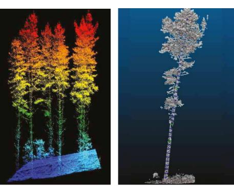
(left) Plot data showing LiDAR collected from a UAV; (right) LiDAR point cloud data for an individual tree where Cloud2stem software has been used to estimate the stem diameter (blue bands)
