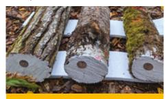
Three bolts each of *Pseudotsuga menziesii*, *Pinus radiata*, and *Notholithocarpus densiflorus* were placed at each field site. Bolts were elevated off the ground with styrofoam panels to avoid soil contact.
