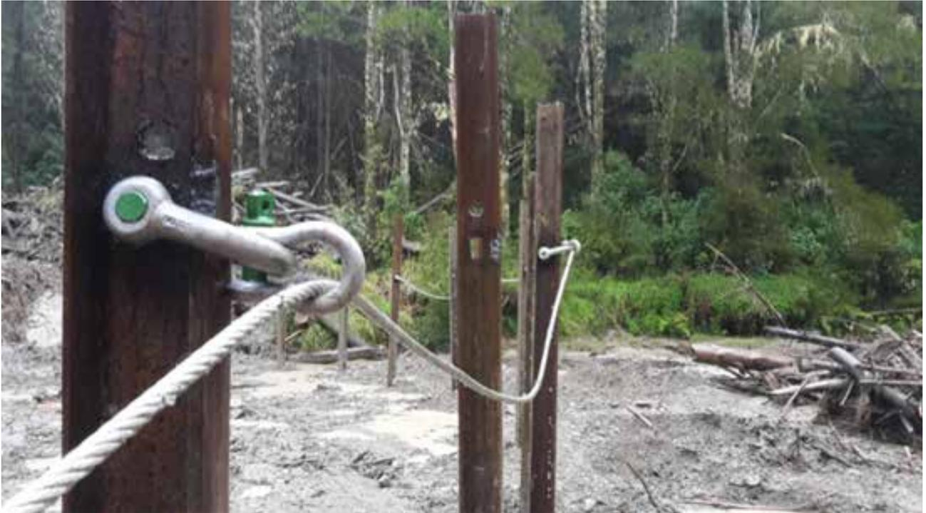
*Rail iron and wire rope slash trap.*
