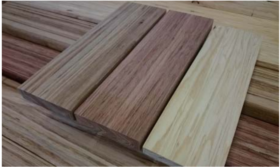
3Wood blocks manufactured from (left to right) Blackbutt, Bluegum and Radiata Pine.
